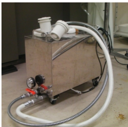
Fig.4.2 Photograph of microbubble device
