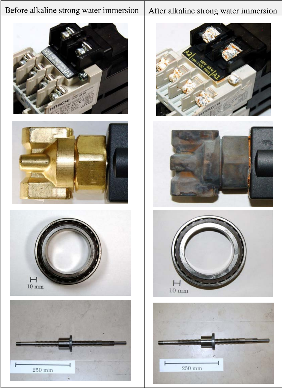
Fig.5.2 Corrosion and discoloration by strong alkaline water
