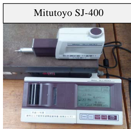
Fig.5.25 Photograph of the surface roughness measuring device
