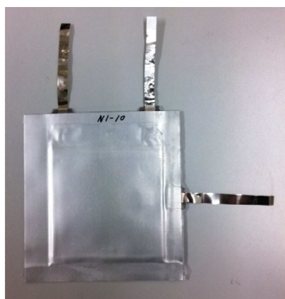
Fig. 2.9 Li-ion cell incorporating a reference electrode.
