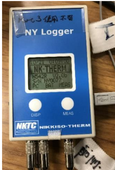
Figure 13: High precision 8-channel data logger
