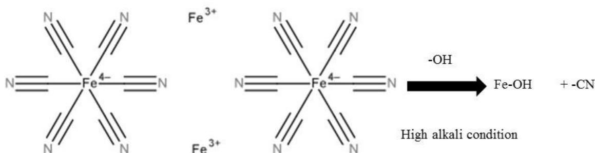
Figure 1-6 Desorption of cyano group from Prussian blue under high alkali image.
