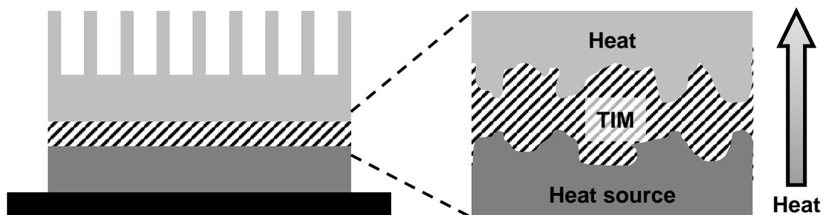
Fig. 1.1 Schematic illustration of Thermal management on electrical devices.
