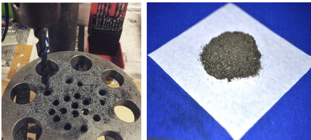
Figure 2.1 Images of cast iron scrap chips generated by the drilling process.
