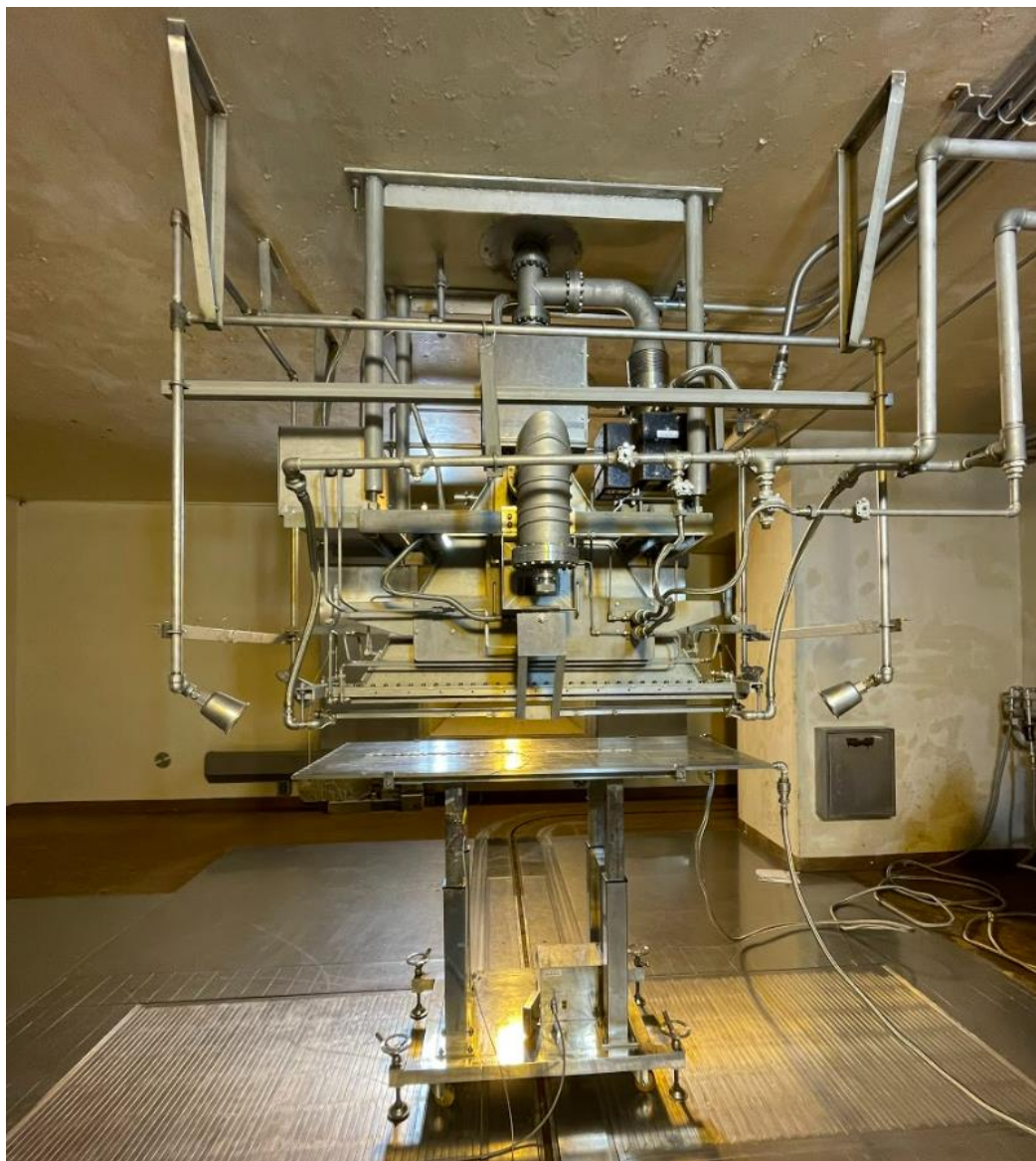
Fig.9 Electron irradiation in the Cockcroft Walton accelerator
