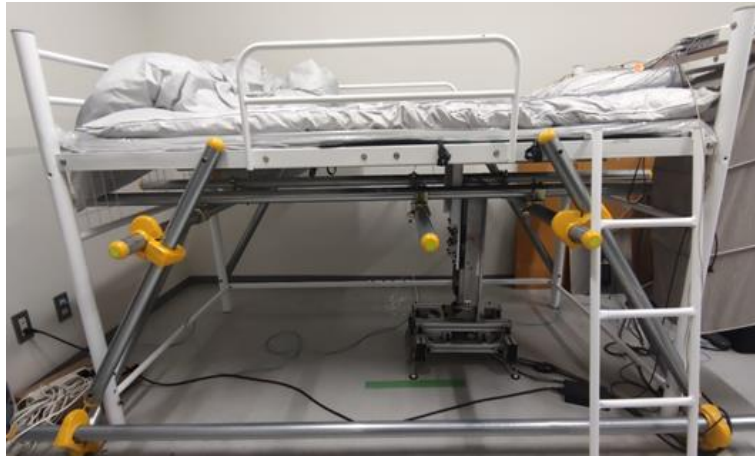
Figure3:Experimental setup used in this study. Participant lied down on a single bed equipped with the lifting device.
