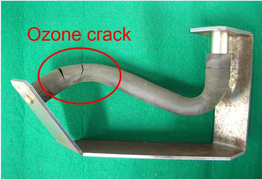
Figure 1-8 Crack propagation of the hose made of NBR used in the oil heater <sup>5)</sup>.
