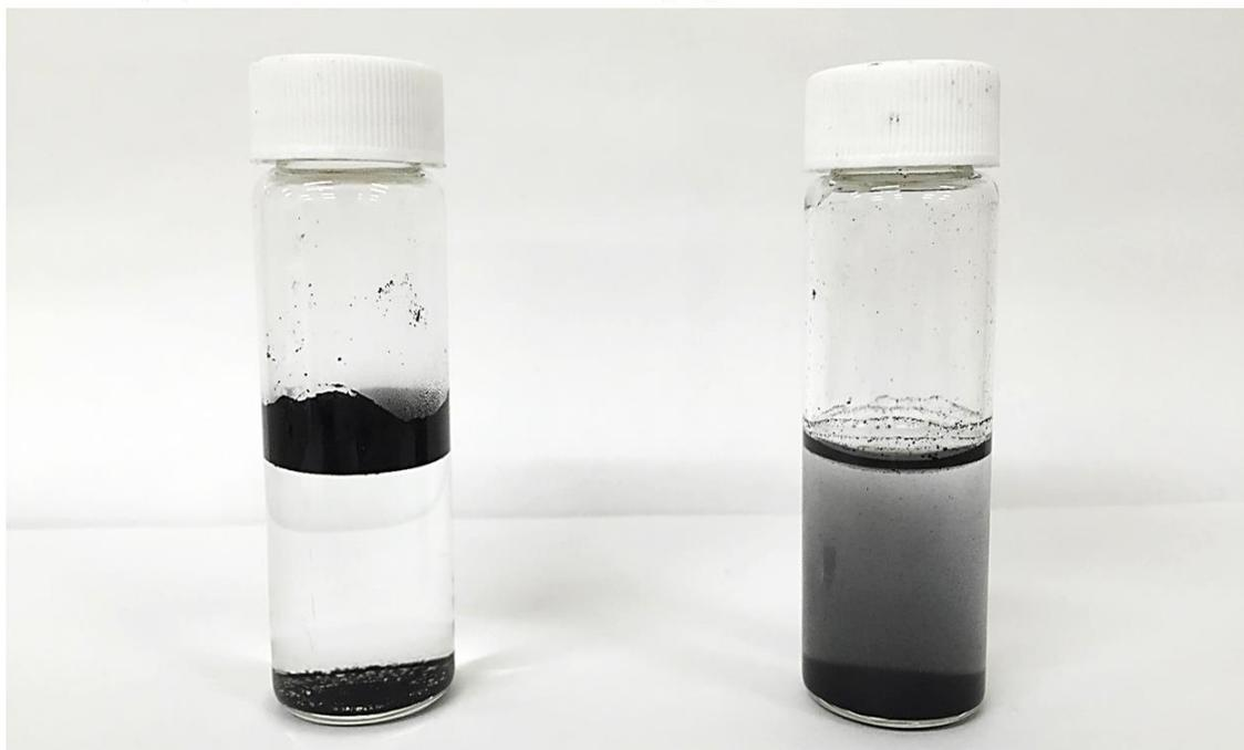
Figure 6-6 The photo images of powder type FT carbon black exposed with (a) air at 80%RH or (b) ozone at 80%RH in ion exchanged water.
