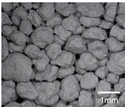
Figure 6-2 Digital microscope images for FT carbon black.
