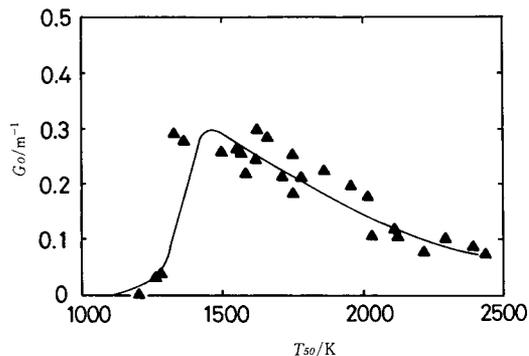
Fig. 10 A comparison between the experimental and calculated dependence of the small-signal-gain on  $T_{50}$  for CO-N<sub>2</sub>O-H<sub>2</sub> system at window I.
