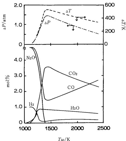
Fig. 9 Calculated concentrations of species and temperature and pressure at  $t = 300 \mu s$  for CO-N<sub>2</sub>O-H<sub>2</sub> system.  $T_{50} = 1500$  K,  $P_{50} = 4.0$  atm.
