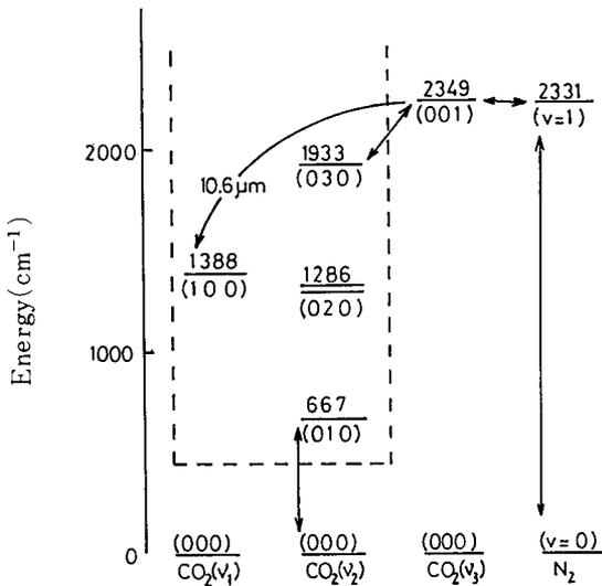
Fig. 3 A vibrational kinetic model for CO<sub>2</sub>-N<sub>2</sub> system<sup>1)</sup>.
