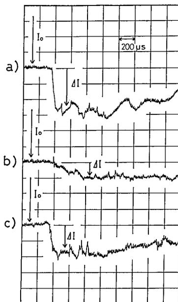
Fig. 5 Comparison of profiles of  $10.6 \mu\text{m}$  small signal gain.
