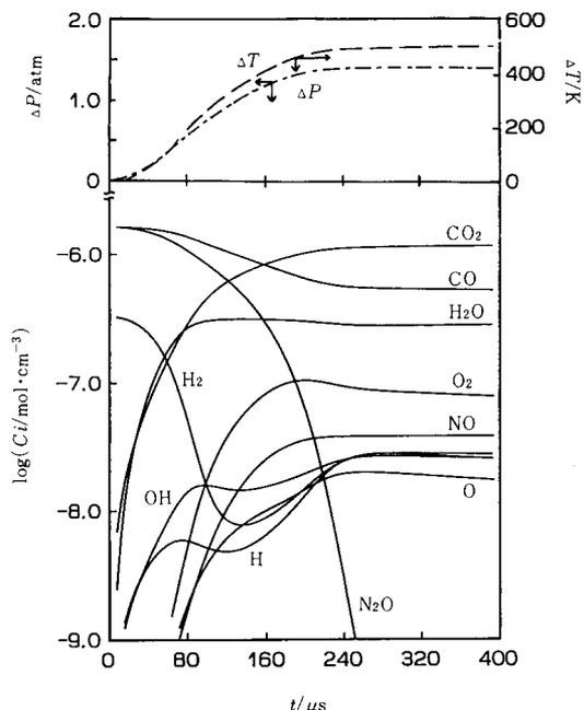
Fig. 8 An example of calculated concentration profiles and temperature and pressure profiles for CO-N<sub>2</sub>O-H<sub>2</sub> system.  $T_{50} = 1500$  K,  $P_{50} = 4.0$  atm.
