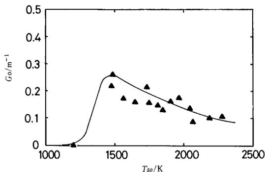
Fig. 11 A comparison between the experimental and calculated dependence of the small-signal-gain on  $T_{50}$  for CO-N<sub>2</sub>O-H<sub>2</sub> system at window II.
