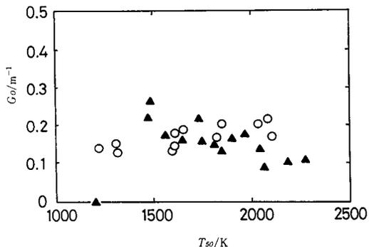
Fig. 7 Temperature ( $T_{50}$ ) dependence of small-signal gain measured at window II,  $P_{50} = 4.0 \pm 0.2$  atm. (○: mixture a, ▲: mixture C)
