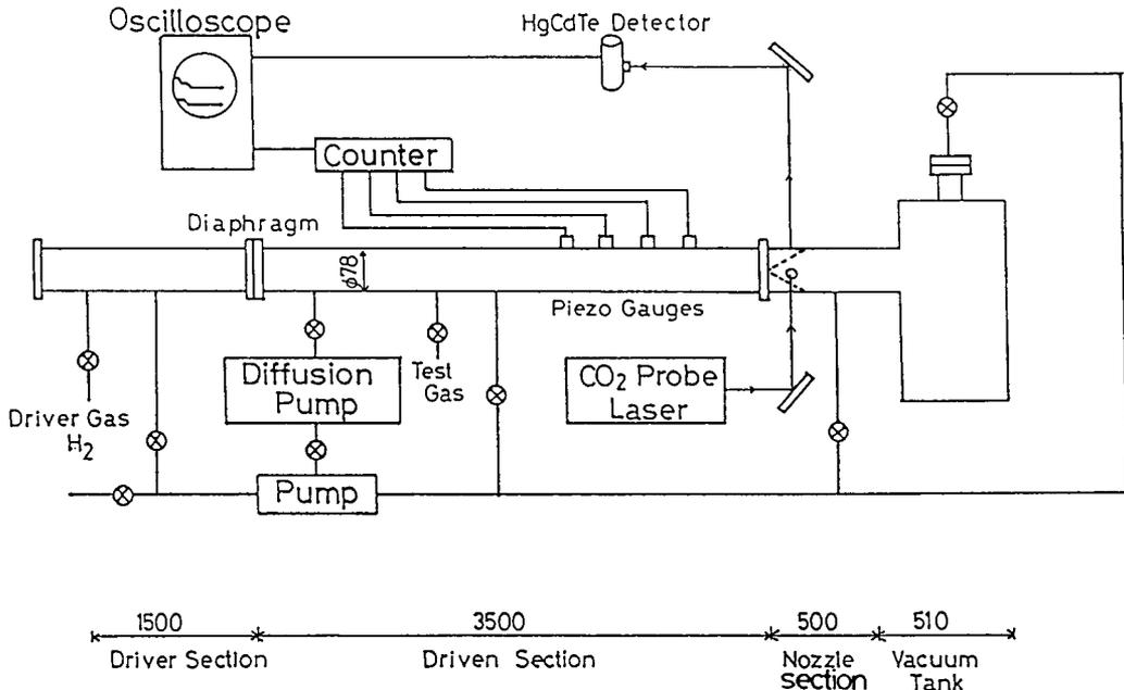
Fig. 1 A schematic of the shock tube for gasdynamic laser experiment.
