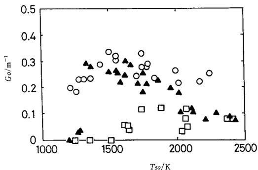
Fig. 6 Temperature ( $T_{50}$ ) dependence of small-signal gain measured at window I,  $P_{50} = 4.0 \pm 0.2$  atm. (○: mixture a, □: mixture b, ▲: mixture C)
