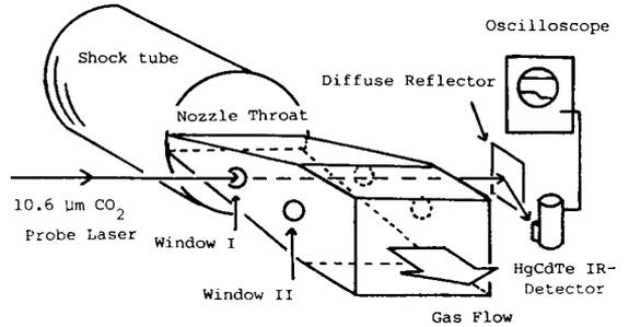
Fig. 2 A schematic of the instrument for gain measurement.
