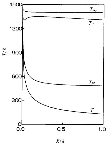
Fig. 4 An example of steady-state vibrational and translational temperature distributions through the nozzle obtained by the numerical simulation.  $T_{N_2}$ ,  $T_3$  are the vibrational temperatures of  $N_2$  and  $\nu_3$ , respectively, and  $T_{12}$  is the combined vibrational temperature of  $\nu_1$  and  $\nu_2$ .  $T$  is the translational temperature. The distance is normalized with the nozzle length  $d$ .  $T_{50} = 1500$  K and  $P_{50} = 4.0$  atm.
