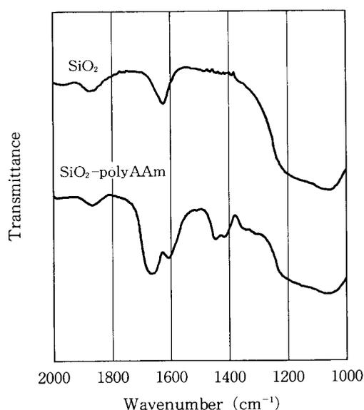
Fig. 3 IR spectra of untreated silica gel ( $\text{SiO}_2$ ) and polyAAm-grafted silica gel ( $\text{SiO}_2$ -polyAAm).
