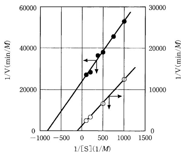
Fig. 6 Lineweaver-Burk plots for the glucose oxidation (at 30°C, pH 7.0) with GOD : ○, native; ●, immobilized on polyAAm-grafted silica gel. The concentration of GOD was 10mg/l.
