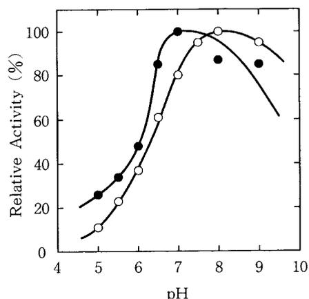
Fig. 4 Effect of pH on the activity (at  $30^\circ\text{C}$ ) of GOD : ○, native ; ●, immobilized on polyAAm-grafted silica gel.
