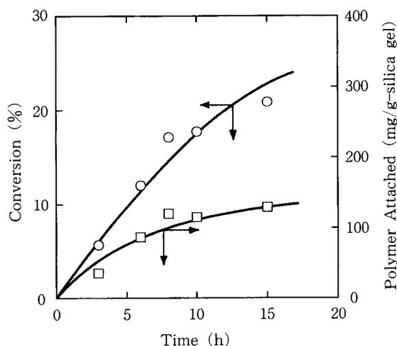
Fig. 2 Polymerization of AAm in the redox system consisting of ceric ion and mercapto groups introduced onto silica gel.
