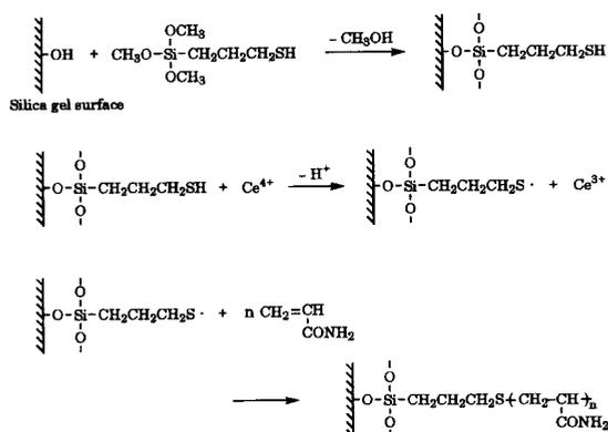
Fig. 1 Grafting of polyAAM onto silica gel surface.
