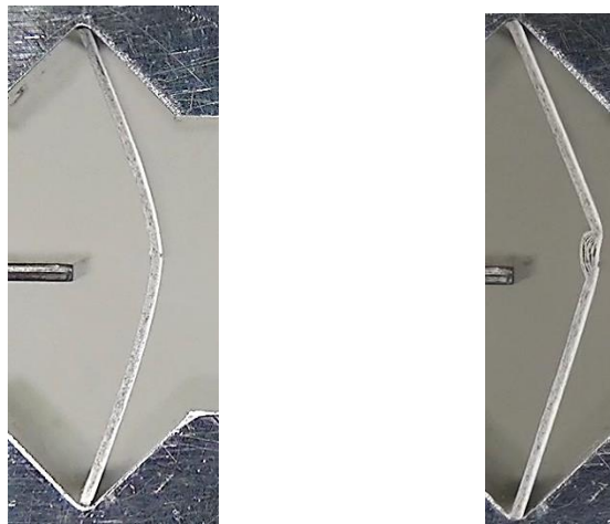
(a) Under compressive test (non-creasing stage) (b) Under compressive test (creasing stage)
