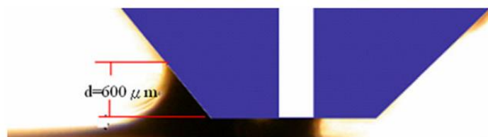
Fig. 2.2 Photo showing the coating bead at the lip of coater. Coater gap is 200 \mu\text{m} 57) .
