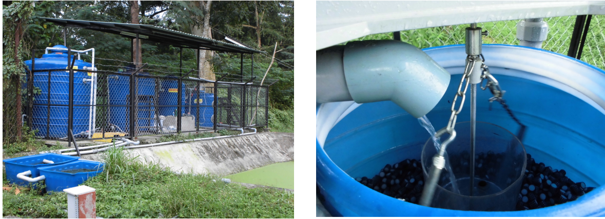
Figure 3.7 Schematic and photo of the pilot scale ABR-UASB-ST-DHS system
