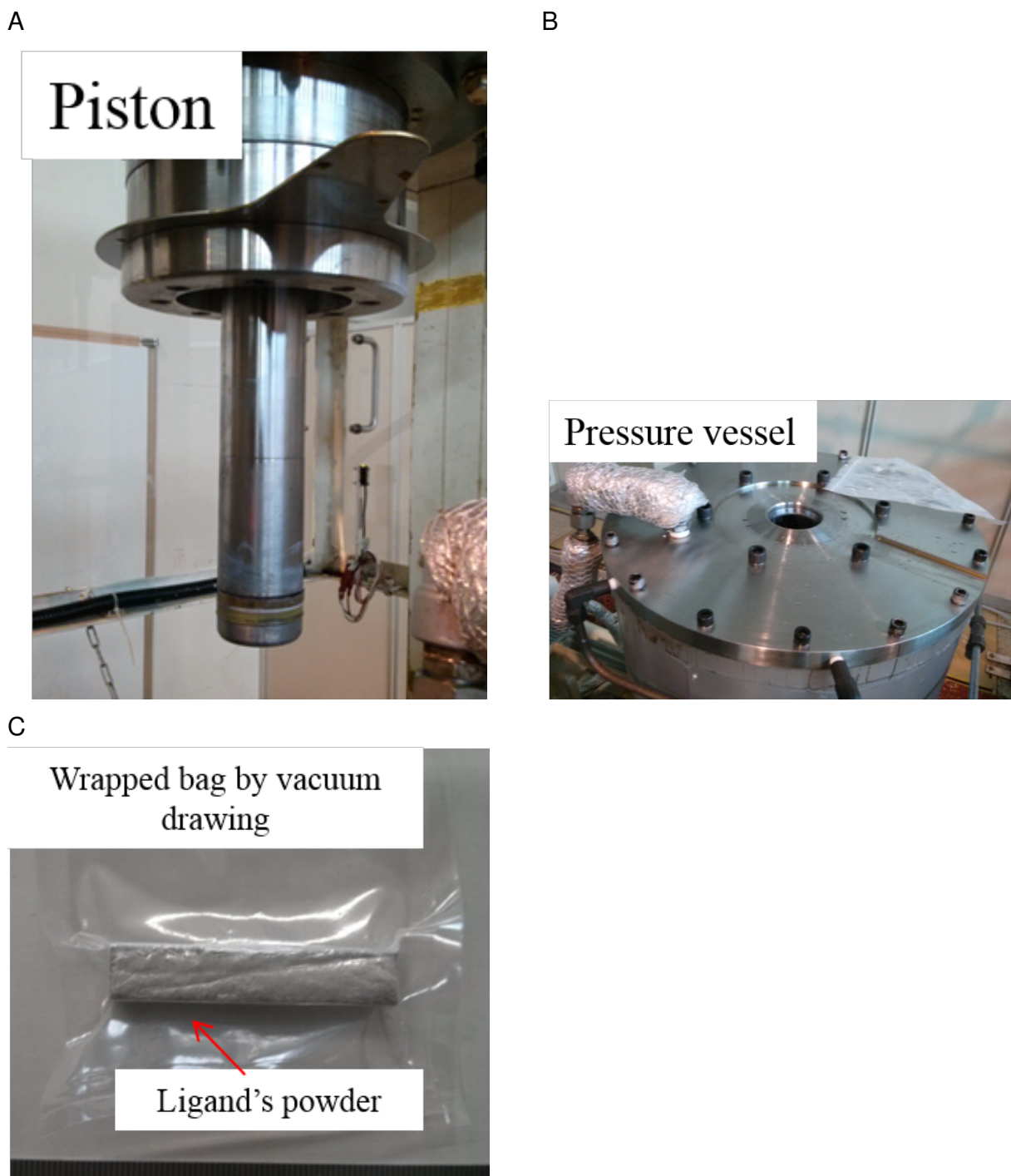
Fig. 2.1 Cold Isostatic Pressing (CIP) machine for fabricating HAp–amino acid complexes. (A)Piston. (B) Pressure vessel which was filled with water. (C) Wrapping samples using a vacuum sealing machine.
