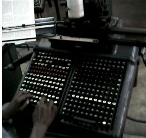
Figure 19: Monotype Composition Keyboard (Courtesy of Sri Lanka Government Printing Department)
