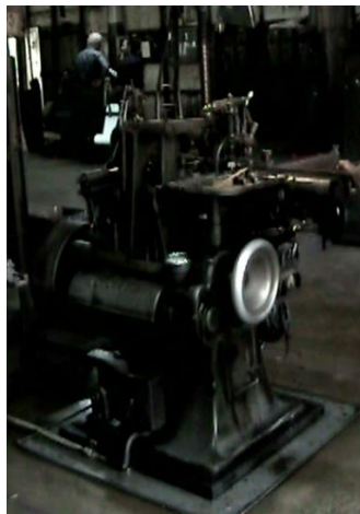
Figure 18: Monotype Composition Caster (Courtesy of Sri Lanka Government Printing Department)
