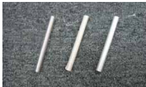
Figure 1. Different kinds of metals (From left: stainless steel, magnesium, aluminum)
