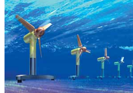
Figure 2. Artist's impression of tidal power generation A system that converts the kinetic energy of tidal currents to power
