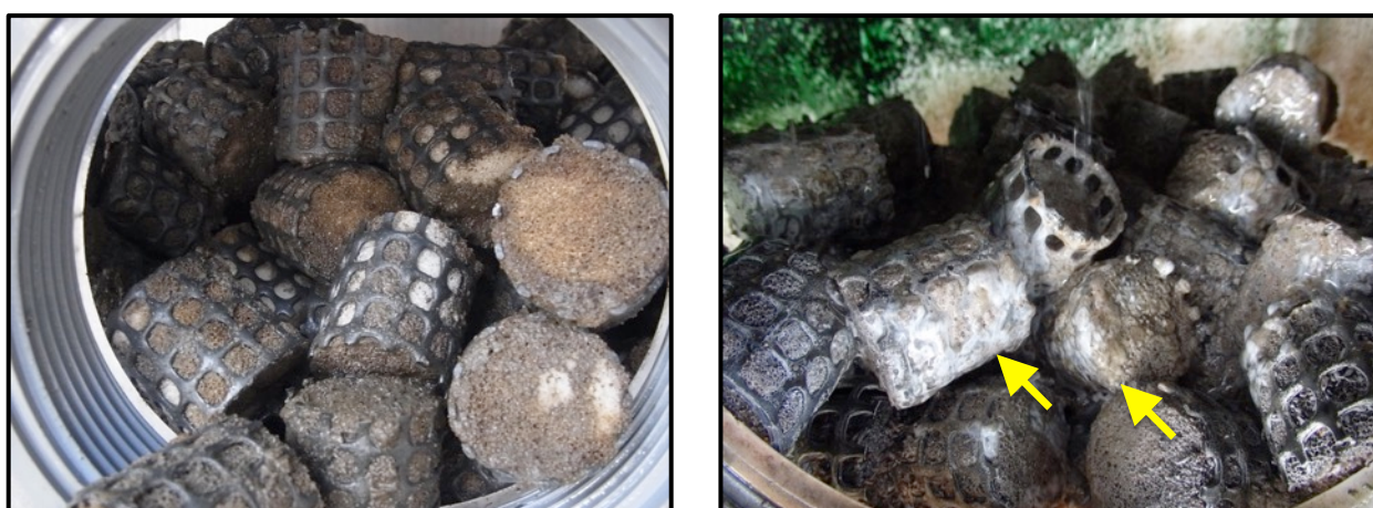
Fig.7-6 Photos of sponge media with retained sludge in the pilot-scale DHS reactor (chapter 6). Left: sponge media with attached retained sludge in general, Right: sponge media with excessively attached retained sludge.
