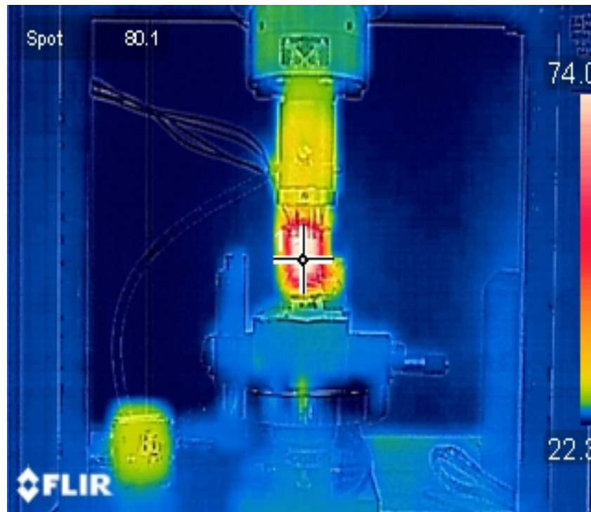
Figure 3-3. Thermographic image of thermal cutting system.
