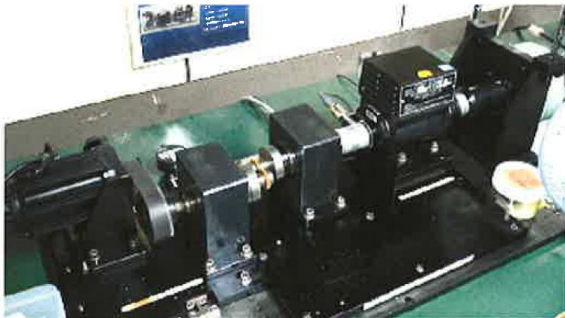
Fig.4-2-2-4 The gear test apparatus
