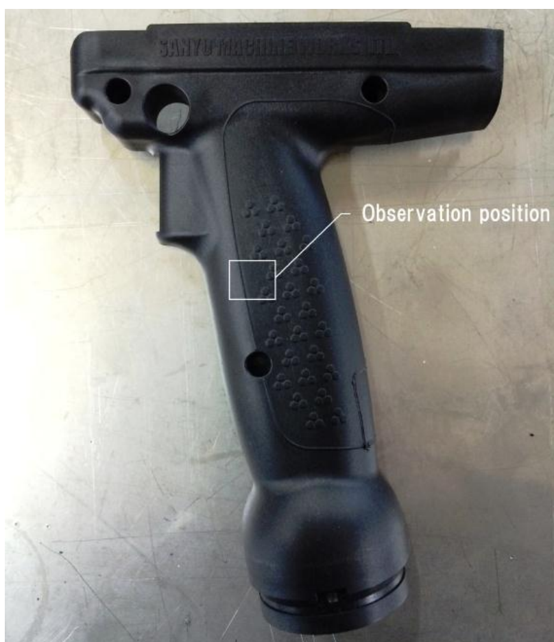
Fig.4-2-1-2 SEM observation position on the surface of electric screwdriver injection molded from GFRPP
