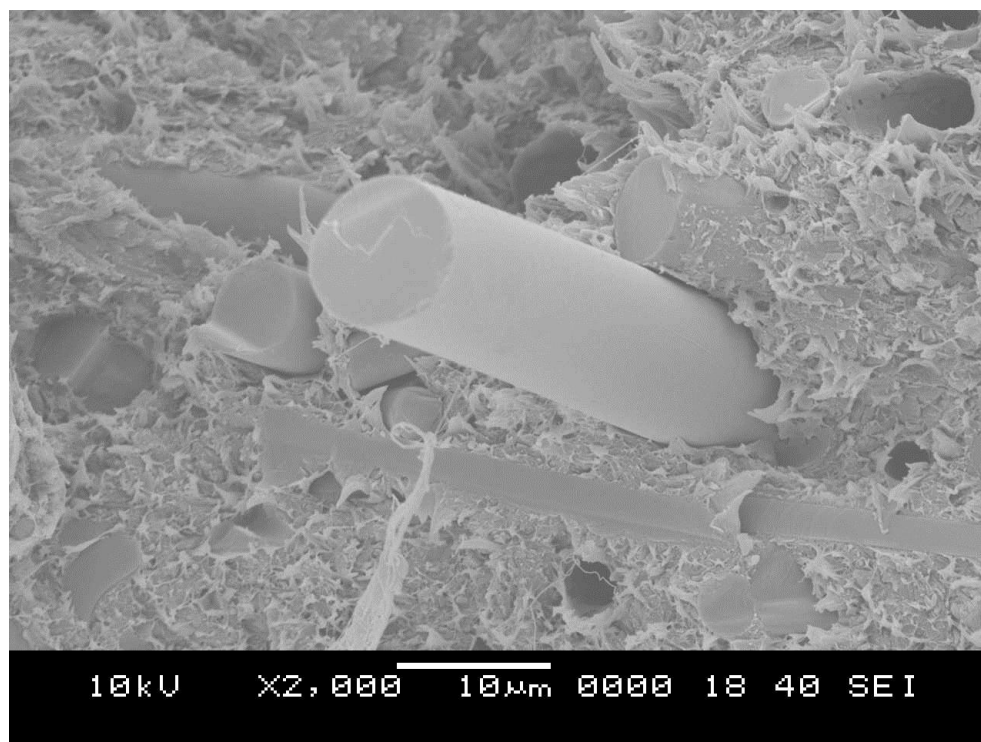
Fig. 2-3-2-4 SEM image of PBT/GW3
