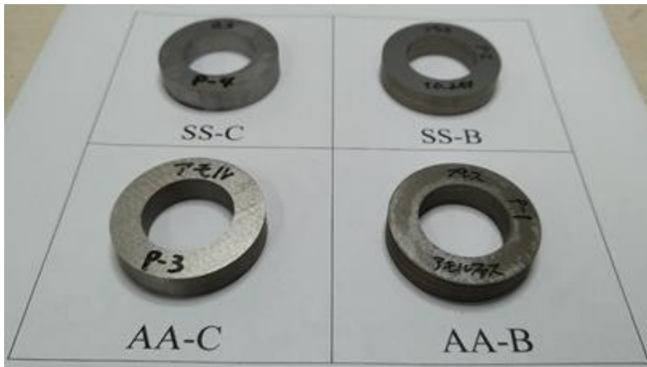
Fig.4.1. Photograph of ring-cores made with the processing methods as shown in Table 4.1.
