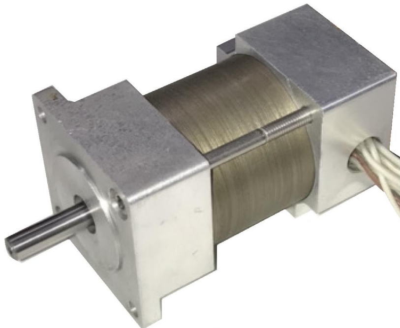
Fig.4.7. Photograph of 70W-SRM made of blanked amorphous alloy foil.
