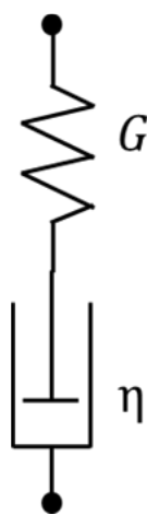
Fig.2.1.6 Schematic of 1D Maxwell model.
